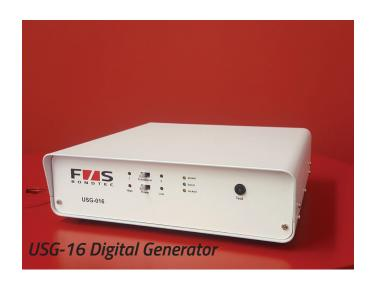
Depending on the operator selection, the digital generator adjusts itself exactly to one of the two operating frequencies of the transducer. This is particularly useful for some components where, for example, bonding is required on package pins. The resonance of such pins can cause bonding problems.
