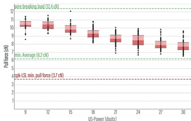
**Figure 3: Pull test results at a bond temperature of 150°C (failure modes: only heel break and lift-off)**
