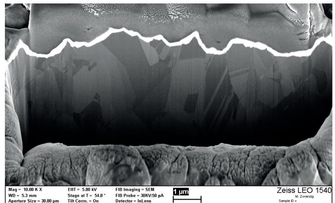
figure 2: FIB-cut into a DIG surface (source: Fraunhofer IZM)
