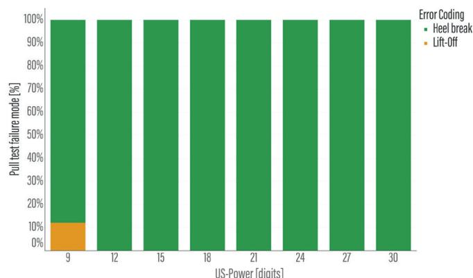
**Figure 4: Distribution of failure modes in the pull test at a bond temperature of 150°C**
