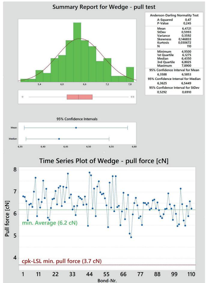
Figure 14: Pull test results wedge  $T_{\text{BOND}} = 20^{\circ}\text{C}$  (RT)
