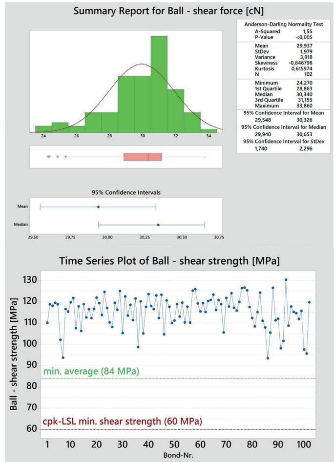
Figure 13: Shear test results ball  $T_{\text{BOND}} = 20^{\circ}\text{C}$  (RT)
