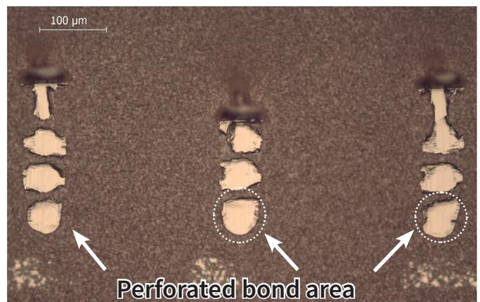
Figure 10: Fracture pattern in shear test (shear-through)
