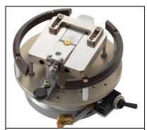
TO workholder with mechanical clamping
